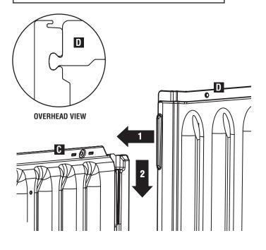
**C** Engage snaps on bottom of **Left Back (D)** into **Repeat Floor (B)**.
